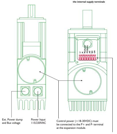
Main power, internal bus voltage and power dump is accessible through these spring contacts placed under the top lid.
