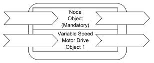
We implement the manufacturer specific variables into Variable Speed Motor Drive functional block, its external name is "ACMotorDrive". Node Object functional block's external name is "NodeObject".
