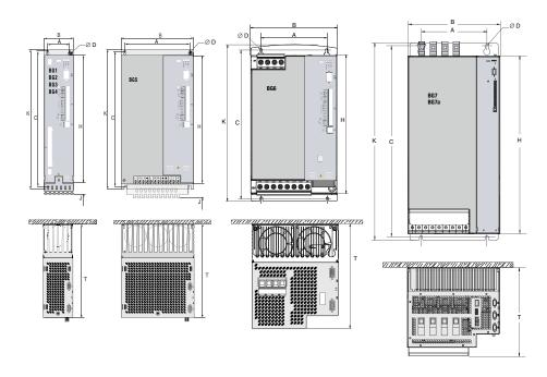
Figure 3.2 Dimensional drawings wall mounting
