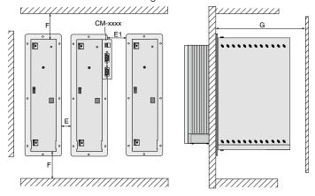
Figure 3.3 Mounting clearances (see Table 3.4)
