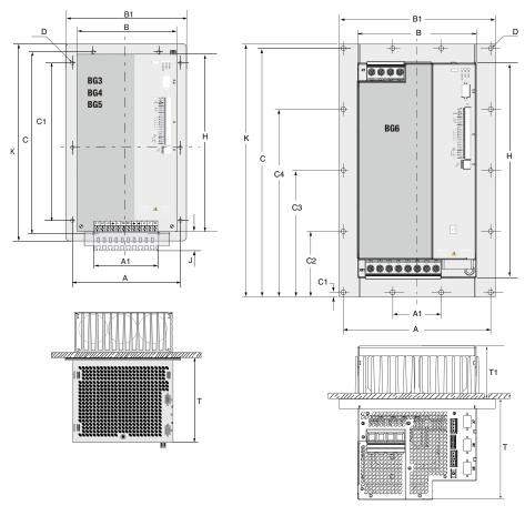
Figure 3.4 Dimensional drawings push-through heat sink (dimensions in mm)
