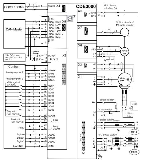
Figure 4.1 Connection diagram CDE3000 (BG1... BG5)
