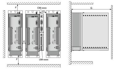
Figure 3.1 Mounting clearances (see Table 3.1)
