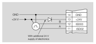
Figure 4.22 Supplying the HTL encoder using an external power supply
