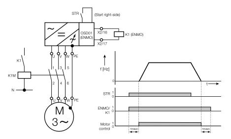
Figure 4.24 Connection example for ENMO. The shield connection is not shown.
