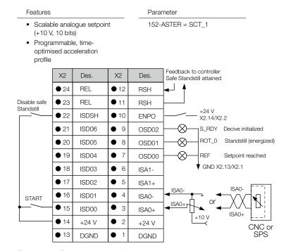
Figure 4.15 Control terminals, drive without encoder evaluation
