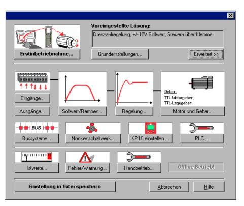
Figure 5.1 Main window for making various settings in DriveManager 3.x
