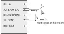
Figure 4.13 Interference on the analogue input with inappropriate wiring
