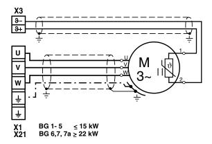
Figure 4.17 Connection of the motor
