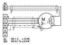
Figure 4.23 Connection of the motor on the CDB3000
