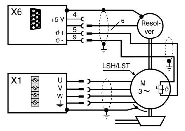
Figure 4.18 Connection of the PTC on LSH/LST motors
