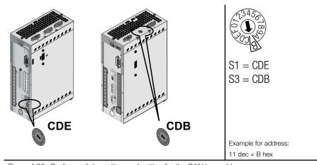
Figure 4.26 Coding switch position and setting for the CAN bus address
