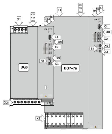
Figure 4.4 Layout of the CDE3000 (BG6, BG7 and BG7a)
