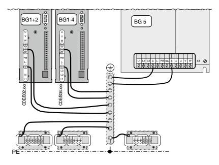
Figure 4.9 Protective earth conductor connection with star topology (BG1-5)
