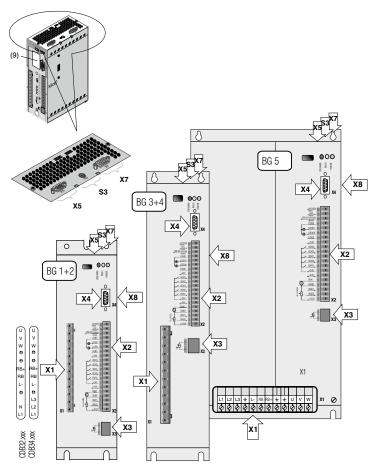
Figure 4.7 Layout DB3000 (BG1 to 5)
