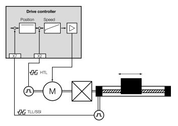
Figure 4.21 Drive with two measuring systems
