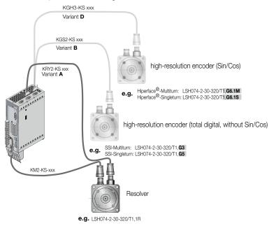
Figure 4.16 Connection of motor/encoder cable to drive controller CDE3000
