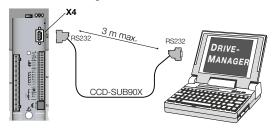
Figure 5.5 Connection of positioning controller to PC/DriveManager 3.x
