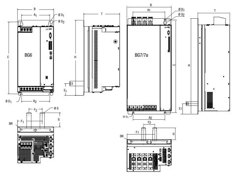
Figure 3.6 Dimensional drawings liquid cooling
