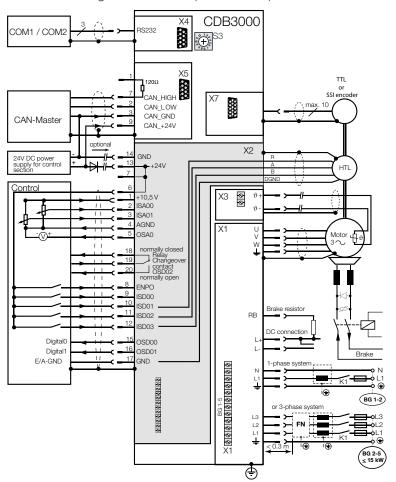
Figure 4.5 Connection diagram CDB3000 (BG1 ...BG5)
