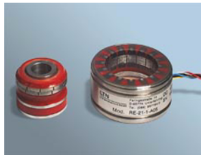
Figure 2.35 Resolver components (source: LTN)
