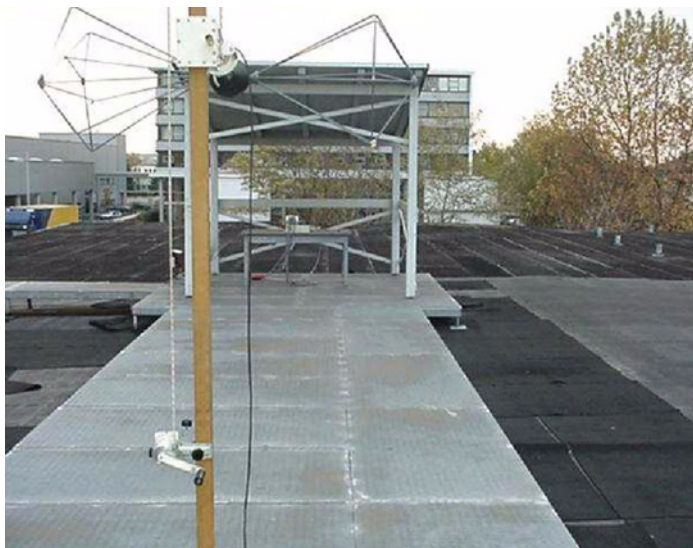
Figure 5.20 Free field measurement of RFI field strength
