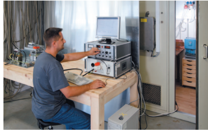
EMC measuring station in front of measuring cabin
