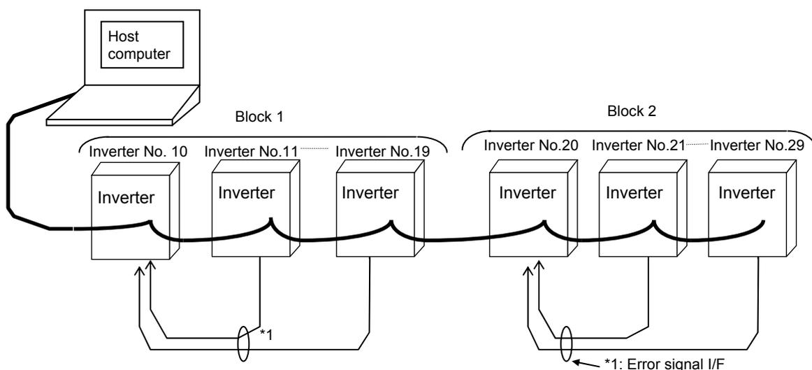
In broadcast communications, only the representative inverter in each block returns data to the host computer. However, you can make the representative inverter in each block report the occurrence of a problem in the block. To do so, follow these steps.
