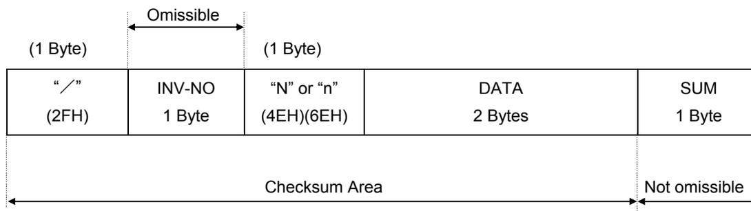
“N” or “n” (1 byte) : Communication error command. Also for check during an inverter trip (includes standing by for retrying and trip holding). “4EH (N)” when normal, “6EH (n)” during an inverter trip.
