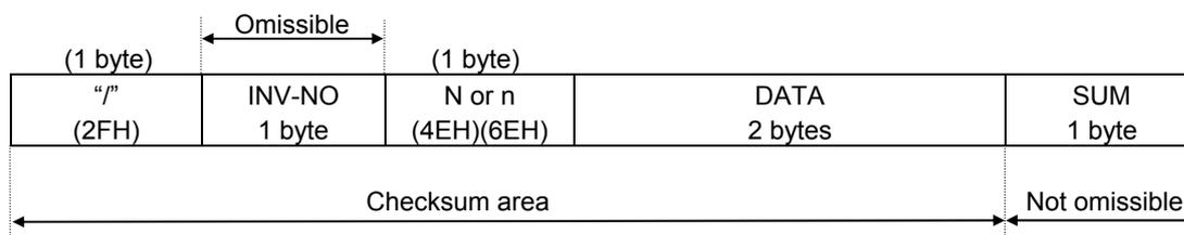
N or n (1 byte) : Communication error command ... This command is also used for a check when the inverter is tripped.
