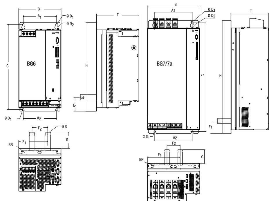
Figure 3.6 Dimensional drawings liquid cooling
