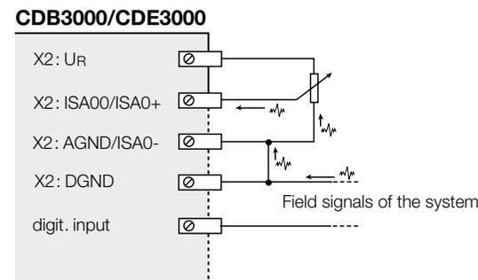
Figure 4.13 Interference on the analogue input with inappropriate wiring
