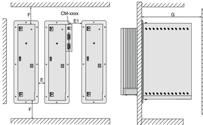
Figure 3.3 Mounting clearances (see Table 3.4)
