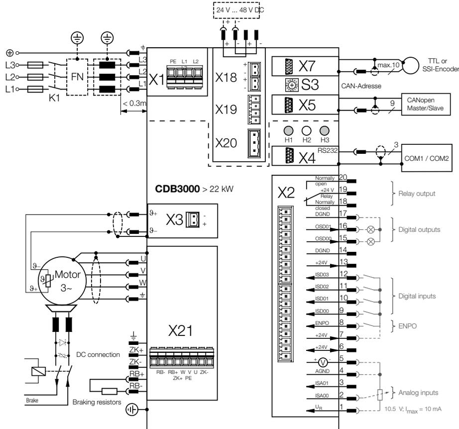
Figure 4.2 Connection diagram CDE3000 (BG6, 7, 7a)
