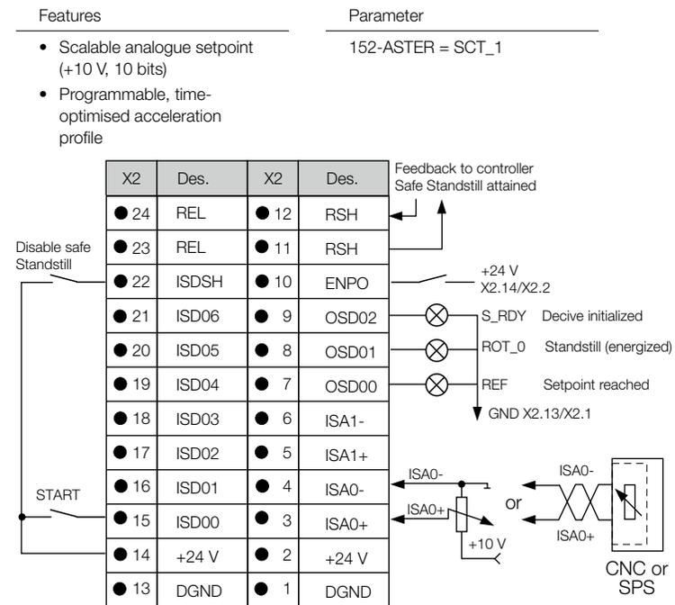
Figure 4.15 Control terminals, drive without encoder evaluation
