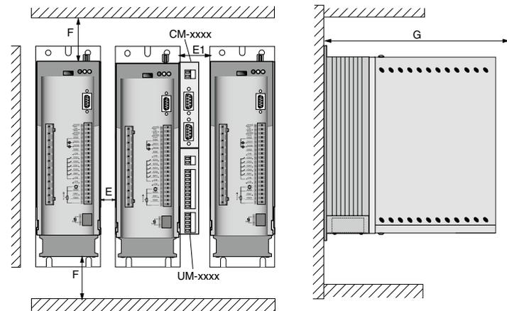
Figure 3.1 Mounting clearances (see Table 3.1)
