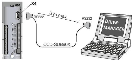
Figure 5.5 Connection of positioning controller to PC/DriveManager 3.x
