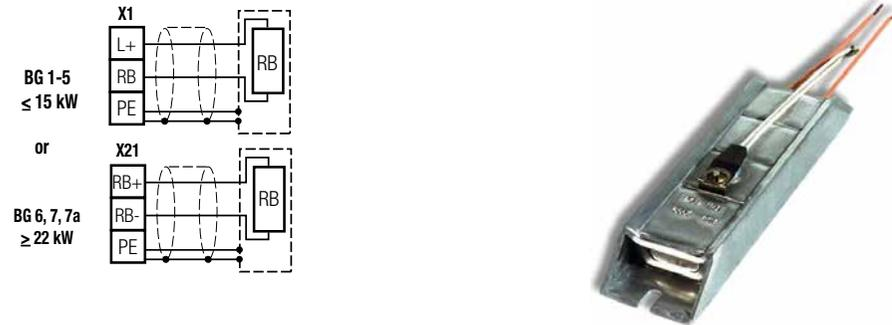
Figure 4.27 Connection of braking resistor
