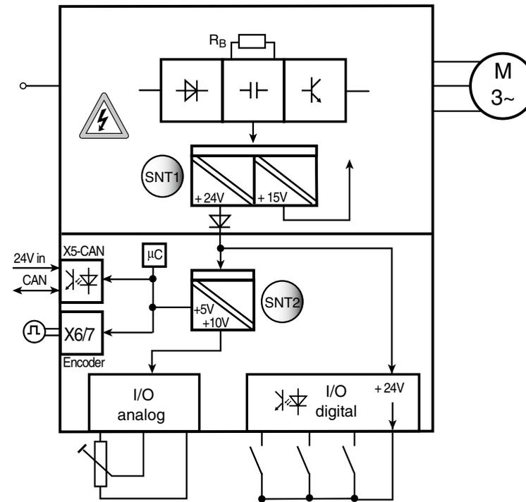
Figure 4.10 Electrical isolation concept/power supply on the CDE3000/CDB3000
