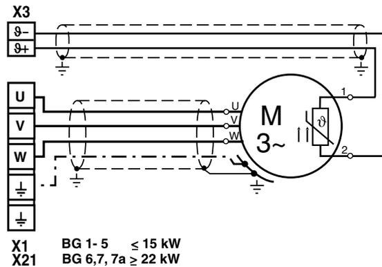
Figure 4.17 Connection of the motor
