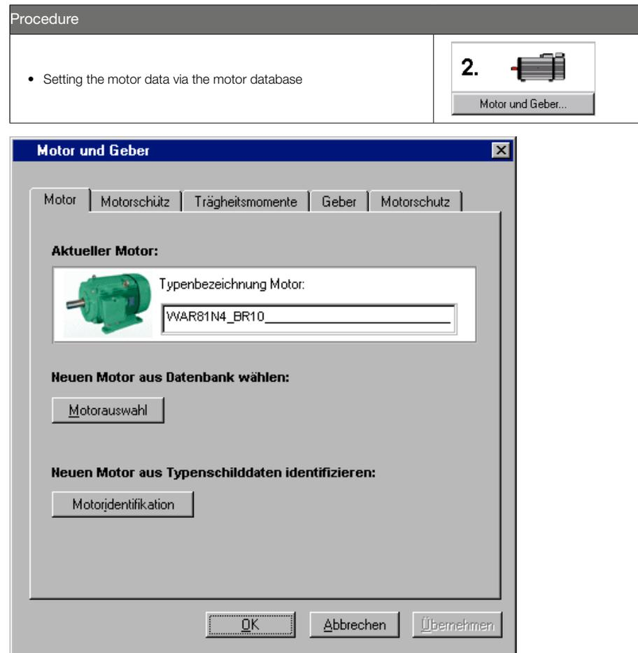
Figure 5.4 Setting motor and encoder
