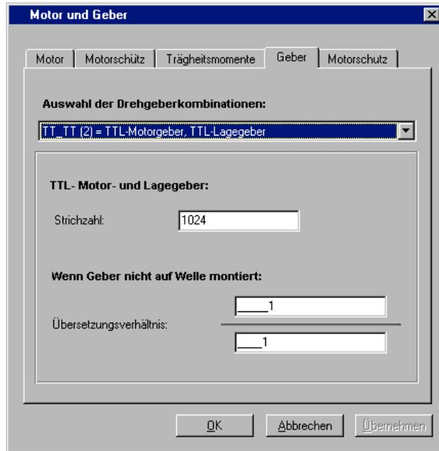
Each encoder combination has a special configuration window.
