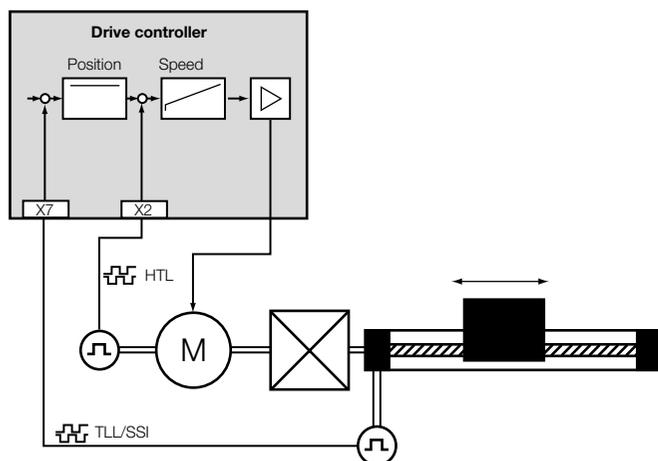
Figure 4.21 Drive with two measuring systems
