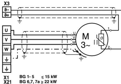
Figure 4.23 Connection of the motor on the CDB3000
