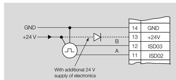
Figure 4.22 Supplying the HTL encoder using an external power supply
