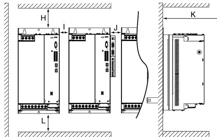
Figure 3.5 Mounting clearances for drive units with liquid cooling
