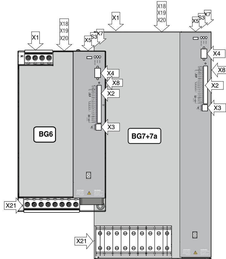
Figure 4.8 Layout DB3000 (BG6, 7 and 7a)
