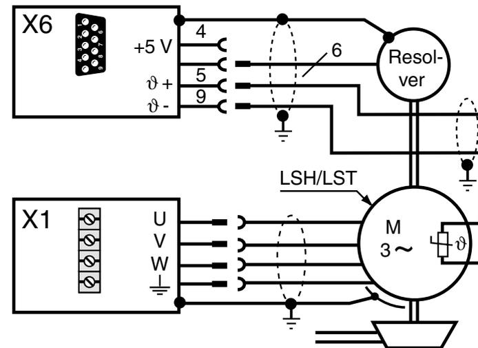
Figure 4.18 Connection of the PTC on LSH/LST motors
