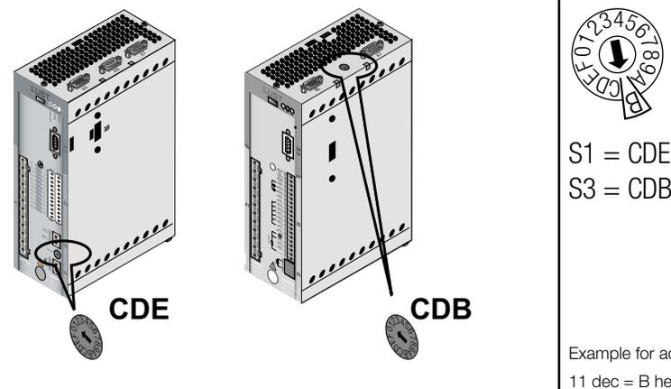
Figure 4.26 Coding switch position and setting for the CAN bus address
